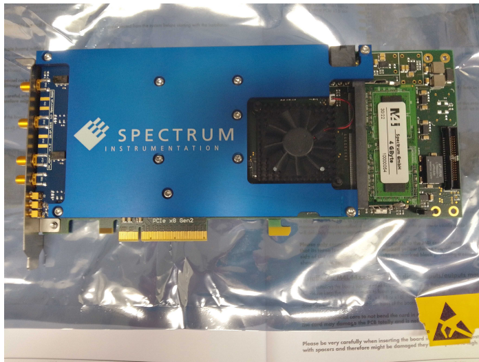
Figure 3.1: Front picture of the AWG placed on the protection foil before installed into the lab PC
